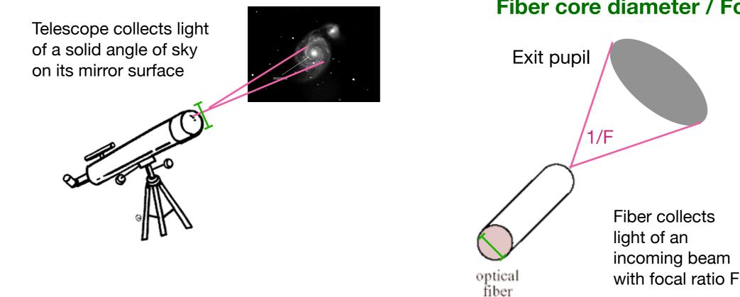
Fiber core diameter / Focal Ratio
