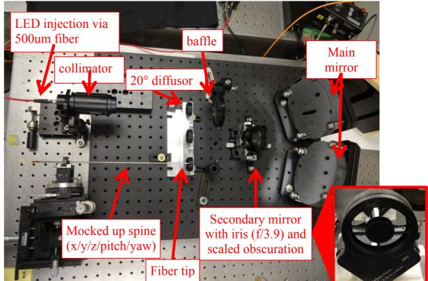
For microlens arrays: measure energy distribution (PSF)
