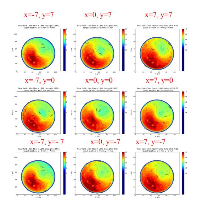
DESI tests demonstrated that on-axis fiber positioners provide stable intensity distribution when a fiber is moved to different positions
